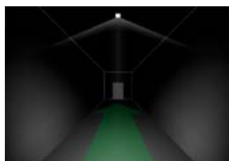
Escape route illumination with symmetric optics
