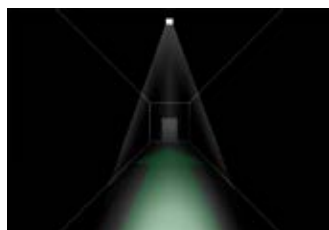
Escape route illumination with asymmetric optics
